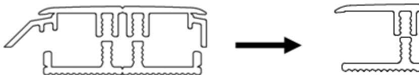
First cut the profile to the correct length. Use the slit to cut away piece X and piece Y to obtain an expansion profile. Then use knife B to slit the profile in half. For installing, gently press the profile from one side of the rail to the other. Press against the floor.
