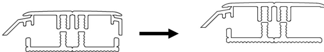
First cut the profile to the correct length. Use the slit to cut away piece Y to obtain an adaptor profile/reducer. For installing, gently press the profile from one side of the rail to the other. Press against the floor.
