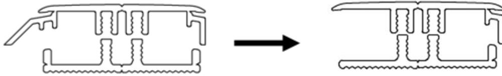
First cut the profile to the correct length. Use the slitser to cut away piece X to obtain a square nose. For installing, gently press the profile from one side of the rail to the other. Press against the floor.
