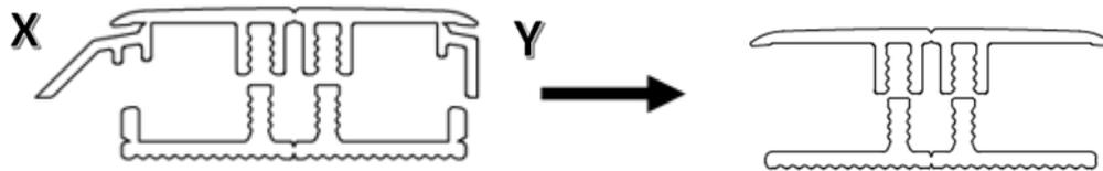
First cut the profile to the correct length. Use the slit to cut away piece X and piece Y to obtain an expansion profile/T-molding. Remark: for easy cutting, cut both lengths before removing the 2 features. For installing, gently press the profile from one side of the rail to the other. Press against the floor.
